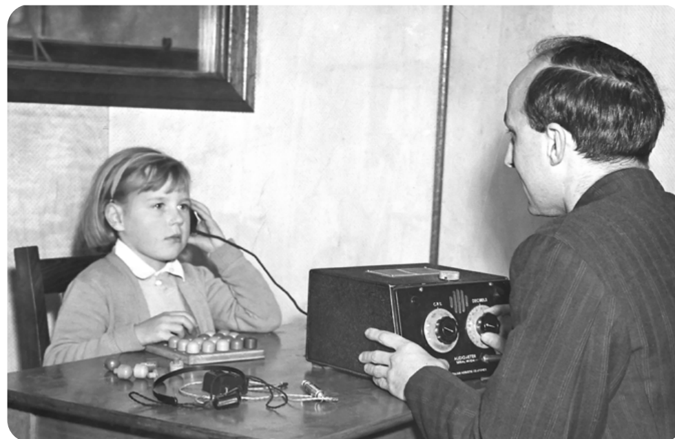
Photo: A pure tone audiometer test of a girl's hearing using a screening audiometer. The test is being carried out by Mr. Roland H. Farrant, Chief Psychologist (now carried out by audiologists) at the Commonwealth Acoustic Laboratory in Melbourne 1949.
